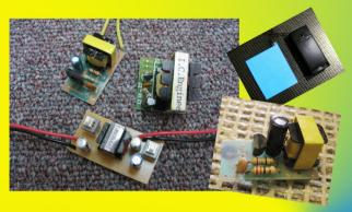
Inverters are a necessary part of any EL project (EL Wire, EL Sheet and any Electroluminescent product). Choose your inverter wisely. Output frequency (Khz or hz) will change the brightness level of your project. Also, some inverters are the blinking type. For examples. Pay close attention the wite length that a particular inverter will run. If you choose an inverter that runs 15 feet of wire, and you attach 30 feet of wire to it, it will be quite dim and the inverter may fail prematurely.
